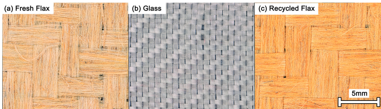
Figure 2. Surface micrographs of the virgin flax (a), glass (b), and recycled flax (c) fabrics.
