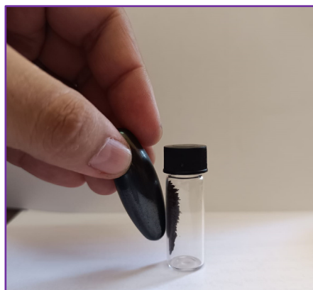
Figure 1. The photograph depicts magnetite nanoparticle powders being drawn to an external magnet.
