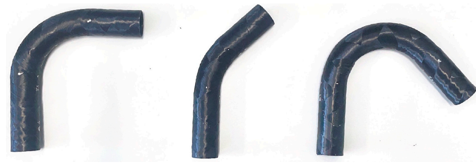
Figure 3. Examples of post-formed CF/PEEK tubes to various bending angles.
