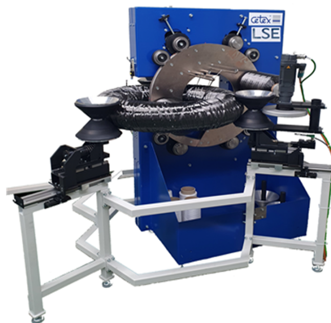
Figure 19. Ring-winding unit of LSE GmbH, designed and manufactured by Cetex Institute GmbH.
