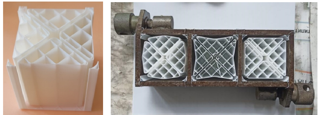
Figure 5. Polymer void former and metal cube mold 70 \times 70 \times 70 mm with installed void formers prepared for molding.
