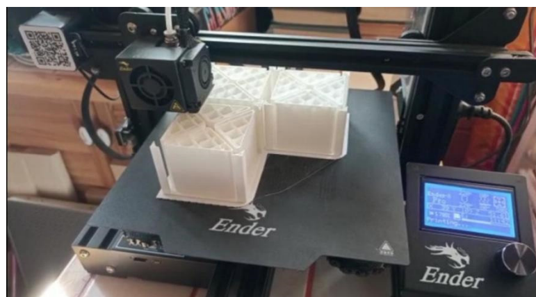
Figure 2. Production of void formers using a 3D printer.
