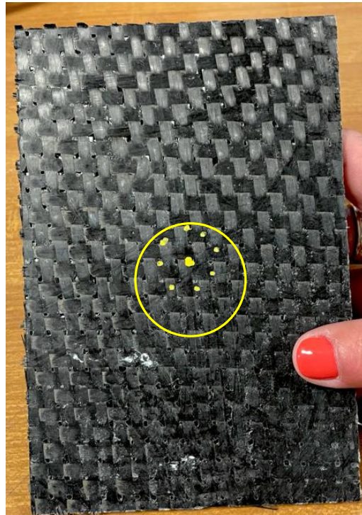
Figure 2. Vent holes and resin injection point on the composite panel.
