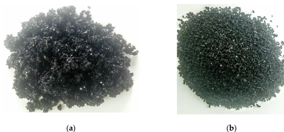
Figure 1. Photos of depleted carbon sorbent: (a)—initial coal sorbent (wet—before drying); (b)—dried sorbent (after drying).
