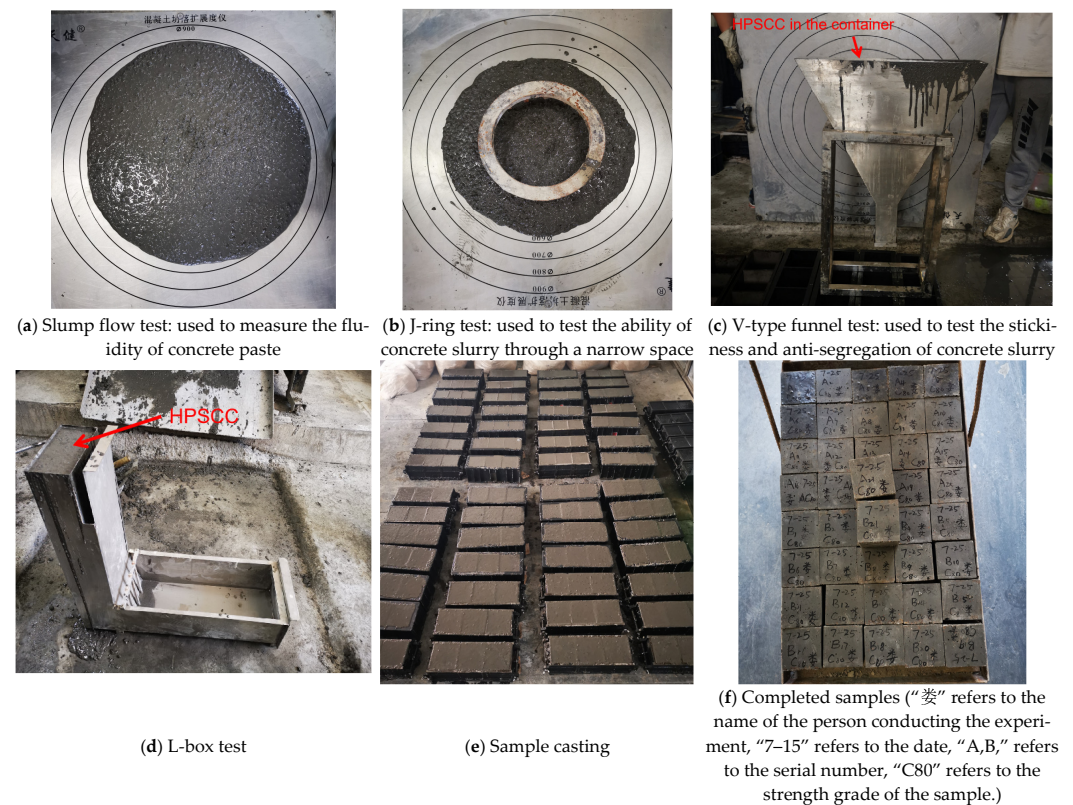
Figure 6. HPSCC experimental samples’ preparation process.
