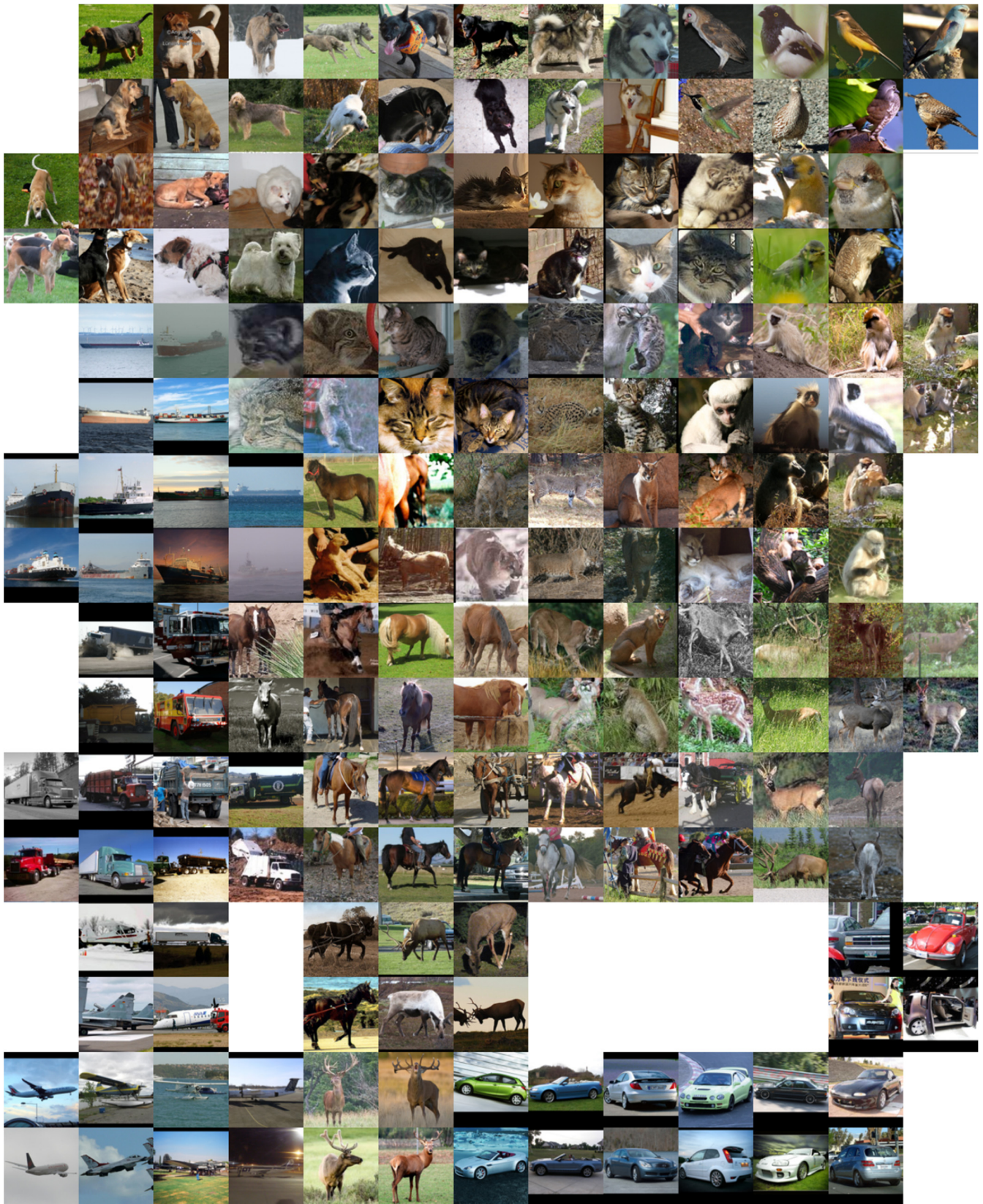
Figure 8. The best-matching images, from the STL-10 testing batch, of every neuron forming the 8 \times 6 SOCOM neural map. Each individual neuron is represented by the four images yielding the highest activations among all the images assigned to the specific neuron. If a neuron describes/contains less than four images (or even no images at all) this is shown by empty/white slots.
