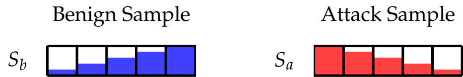
Figure 2. In this synthetic motivating example, we show the disadvantages that can arise when using aggregate loss metrics for detecting anomalies. On the left-hand side, we show the autoencoder feature residuals for a benign network flow sample, while the right-hand side shows the autoencoder feature residuals for an attack. The error for both samples is equal; however, it is distributed differently among the features. An aggregate metric such as mean-squared error would calculate the anomaly score the same for both samples, resulting in the benign sample being flagged as a false-positive. Providing the autoencoder feature residuals to a downstream classifier provides the classifier with the opportunity to differentiate the two samples.
