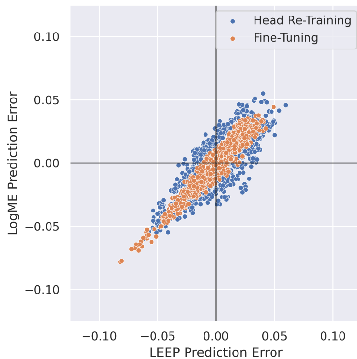
Figure 9. The error in the predicted post-transfer accuracy using a linear fit to the LEEP scores (x-axis) and LogME scores (y-axis) for the sweep over FO. Note the change in scale compared to Figures 8 and 10.
