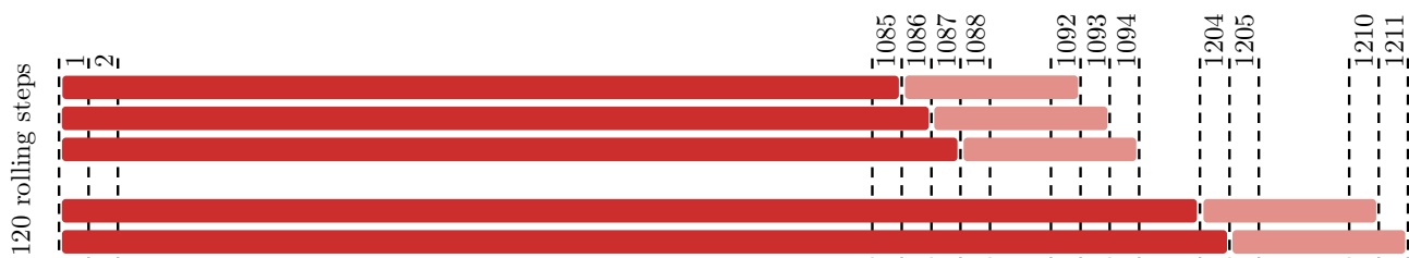
Figure 4. Rolling-window approach for forecasting with 120 rolling steps. The training set is represented by dark-red bars and the testing set by light-red bars. At each step, the training set is incrementally extended by one day, producing forecasts for a 7-day horizon.
