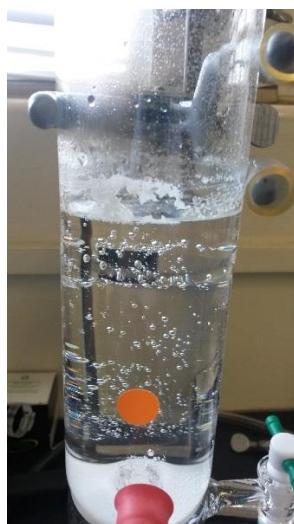
Figure 3. Scum concentrating on the solution surface and adsorbing to the column while floating \text{La}^{3+} at \varphi = 2 .
