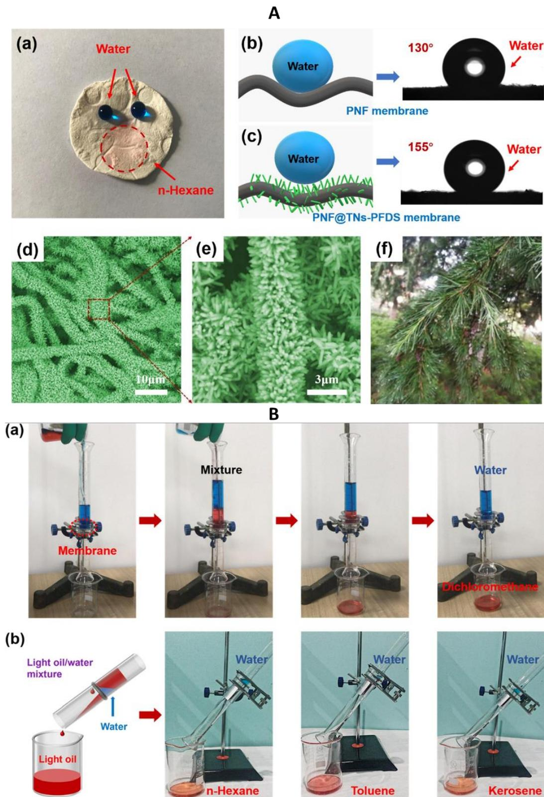
**Figure 8.** (A) (a) The state of water droplets and oil droplets (n-hexane) on the surface of the PNF@TNs-PFDS, the water, and the oil droplets were dyed to blue and red, respectively; (b) The WCA of PNF membrane; (c) PNF@TNs-PFDS fiber membrane; (d,e) SEM images of robust pine needle-like TNs; and (f) Photograph of pine needle. (B) Oil/water separation process of (a) heavy oil and (b) light oil [122]. Reprinted with permission from Ref. [122]. Copyright 2021 Elsevier B.V. All rights reserved.
