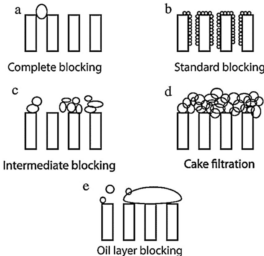
**Figure 1.** Schematic representation of the different fouling mechanisms taking place on the membrane surface [53]. Reprinted with permission from Ref. [53]. Copyright 2016 Elsevier Inc. (Amsterdam, The Netherlands). All rights reserved.
