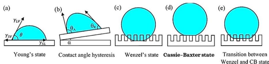
**Figure 2.** Various states of a water droplet on a solid surface [70]. Reprinted with permission from Ref. [70]. Copyright 2020 American Chemical Society.
