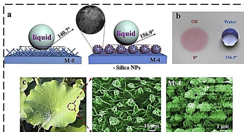
**Figure 6.** (a) Diagrams illustrate the effect of bottom surface structure of M-0 and M-4 on the hydrophobic; (b) Photograph of pure water and oil droplets on the M-4 bottom surface; (c) Optical photograph and SEM image of lotus leaf [119]. Reprinted with permission from Ref. [119]. Copyright 2019 Elsevier B.V. All rights reserved.
