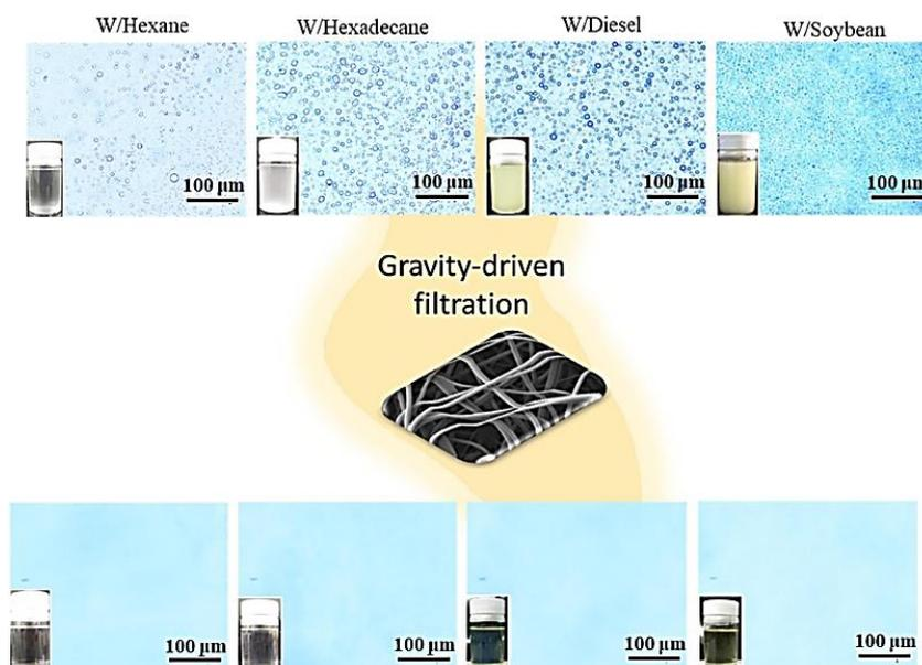
**Figure 7.** Optical micrographs of the feed emulsions (top part) and permeates (bottom part) using PMMA/60PDMS nanofibrous membrane under the sole influence of gravity [121]. Reprinted with permission from Ref. [121]. Copyright © 2023 Elsevier B.V. All rights reserved.
