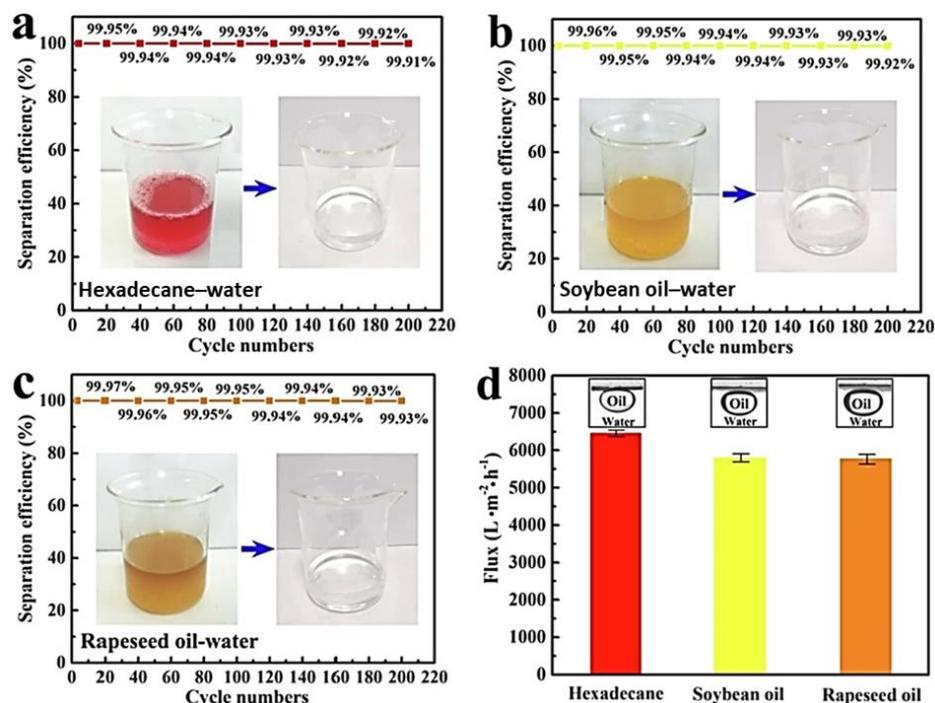
**Figure 10.** Separation efficiencies of CuO@PAA membrane for various oil–water combinations (a–c) and water penetration fluxes (d). Insets 10a, b, and c show oil–water combinations and filtered water; 5d shows hexadecane, soybean oil, and rapeseed oil on CuO@PAA membrane in water [139]. Reprinted with permission from Ref. [139]. Copyright © 2023 Elsevier B.V. All rights reserved.
