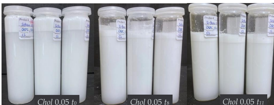
Figure S1: Images of the Ref samples cooled at a slow (0.01–0.1 K/min, left flask), moderate (0.5 K/min, middle flask) or fast (10 K/min, right flask) rate, taken at t_0 , t_8 and t_{11} .
