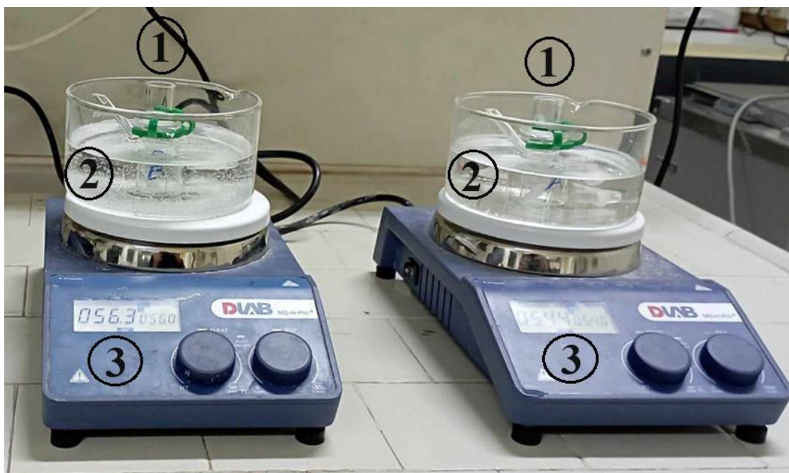
Figure S3 (Supplementary data): Franz cell assembly for in vitro diffusion study of voriconazole: (1) Franz cell diffusion system; (2) Water bath; (3) Magnetic stirrer
