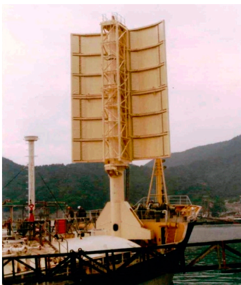
Figure 4. Japan Machinery Development Association (JAMDA) Rigid Sail at Teramoto Iron Works in the 1980's [47].
