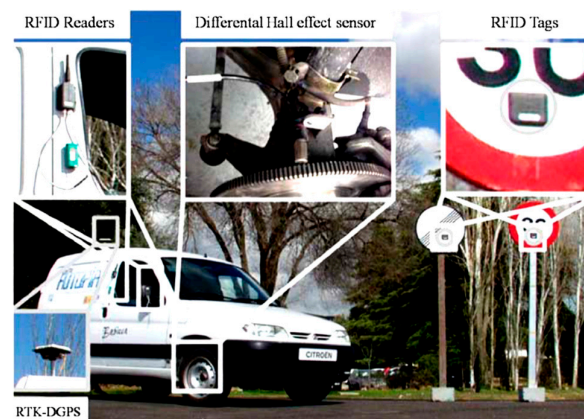
Figure 21. A depiction of the various sensors deployed on a car for experimenting [57].
