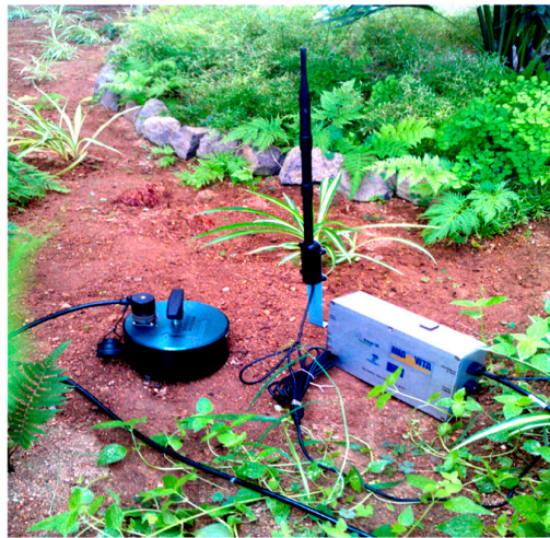
Figure 11. A depiction of a geophone sensor with a wireless antenna deployed in the field [23].
