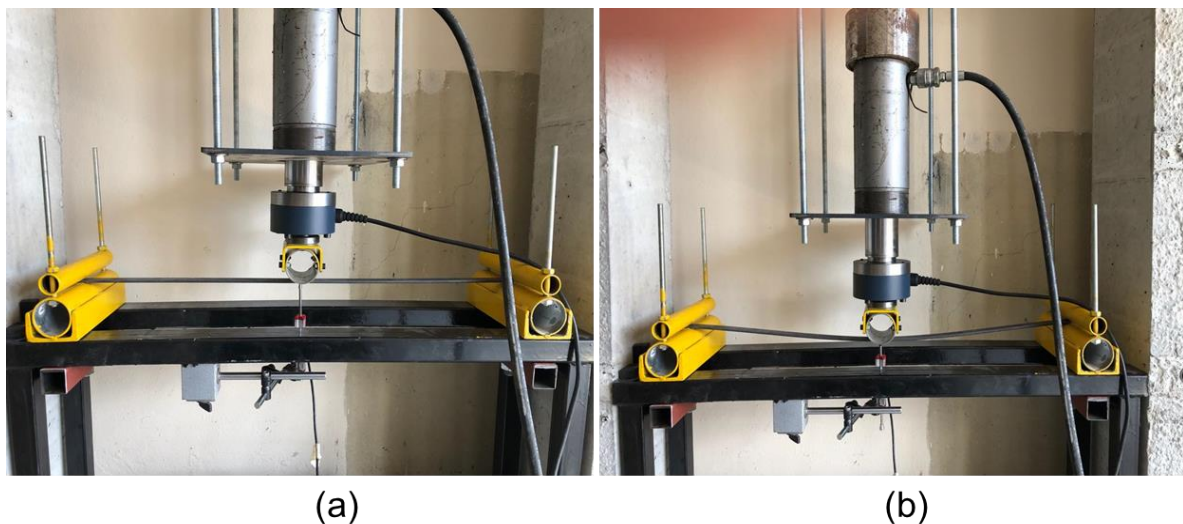
Figure 2. Testing the response of the control specimens under quasi-static testing (a) during testing and (b) after testing.
