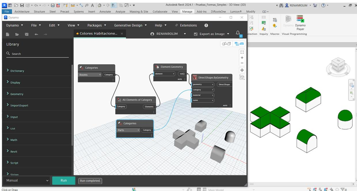
**Figure 12.** Materialisation in Revit of the interiors of simple shapes using the Dynamo plug-in. In this case, it is possible to visualise them in both Revit and Dynamo. Source: own elaboration (2024).
