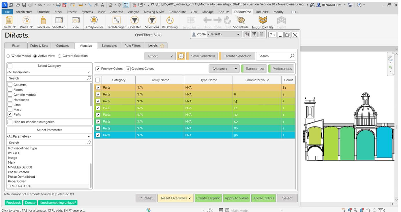
Figure 15. Visualisation of the heat map in Autodesk Revit 2024 using the DiRoots plug-in filter. On the left, filters applied in DiRoots to detect the parameters inserted into the internal spaces materialised as 'pieces'. On the right, visualisation in Revit of the heat map in the 2D section. Own elaboration (2024).
