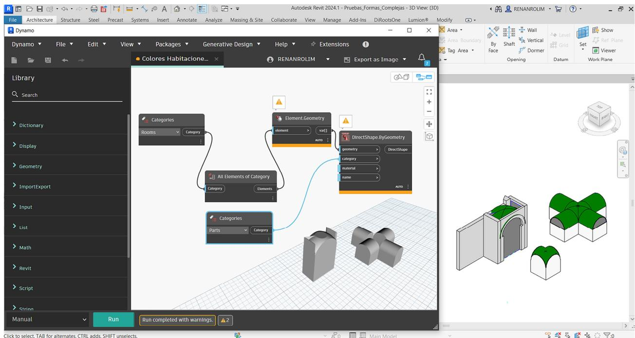
**Figure 13.** Materialisation in Revit of the interior spaces of complex shapes using the Dynamo plug-in. In this case, it is only possible to visualise some types of errors in Dynamo. Source: own elaboration (2024).
