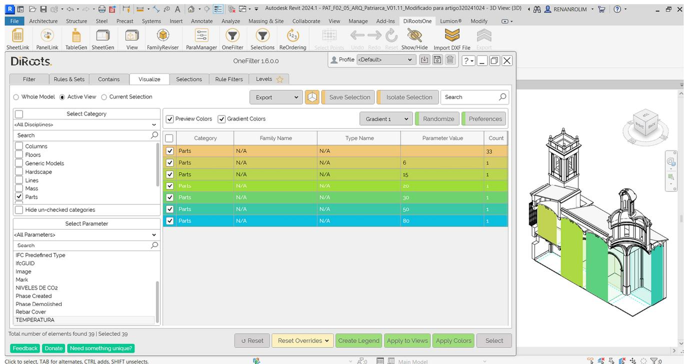
**Figure 16.** Visualisation of the heat map in Autodesk Revit 2024 using the DiRoots plug-in filter. On the left, filters applied in DiRoots to detect the parameters inserted into the internal spaces materialised as ‘pieces’. On the right, visualisation in Revit of the heat maps in the three-dimensional section. Own elaboration (2024).
