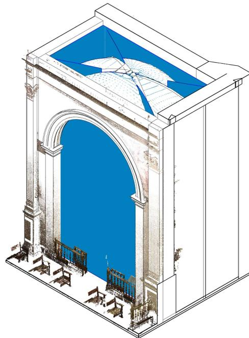
**Figure 9.** Materialisation of the interior spaces of a side chapel using the Autodesk Dynamo plug-in. In blue: materialised volume with errors in the connections between the plementeries and between the plementeries and the walls. Source: own elaboration (2024).
