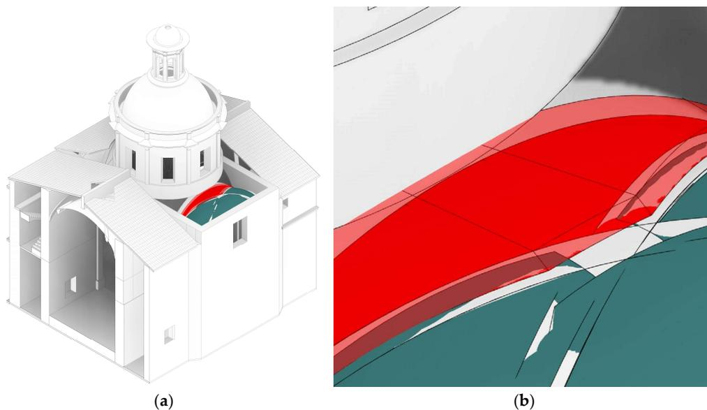
**Figure 6.** Error in the extrusion of the mass layer. (a) In green: plementeries modelled with the mass tool; in red: error presented in the plementeries when the extrusion was performed on the created mass; (b) detail focused on the error presented in the plementeries. Source: own elaboration (2024).
