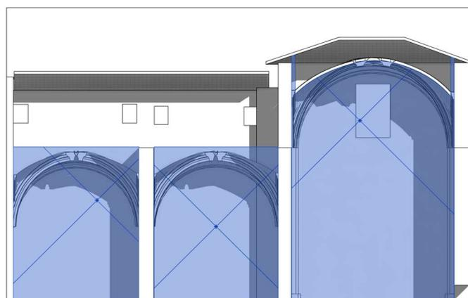
**Figure 8.** Visualisation of the vaults using the 2D section in Revit 2024, demonstrating that the mass surfaces that allowed for the conversion to the roof now limit the height of the spaces. Centre and left: mass surfaces that did not allow conversion; right: mass surfaces that allowed conversion but still required manual adjustments. Source: own elaboration (2024).
