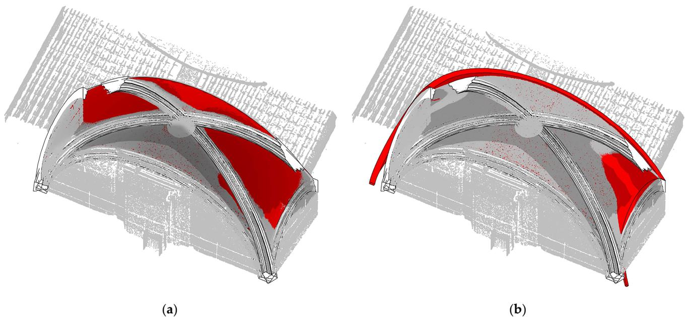
**Figure 10.** Overlay of the point cloud (in grey) and the 3D model (in red) of the vault showing the geometric divergence between the modelled vault and the point cloud. It can be seen that the vault modelled separately as a mass layer (a) is visibly more accurate than the vault modelled as a single element (b). Source: own elaboration (2024).
