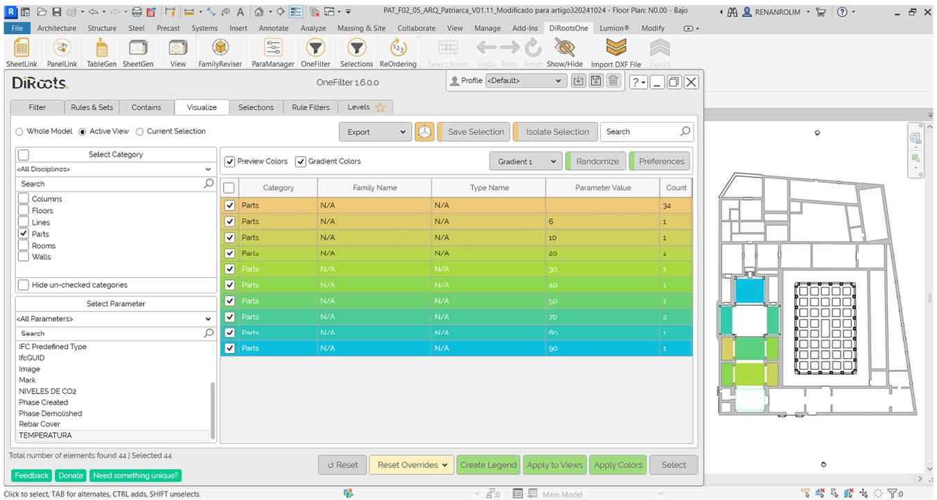
Figure 14. Visualisation of the heat map in Autodesk Revit 2024 using the DiRoots plug-in filter. On the left, filters applied in DiRoots to detect the parameters inserted into the internal spaces materialised as 'pieces'. On the right, visualisation in Revit of the heat map on the ground floor. Own elaboration (2024).
