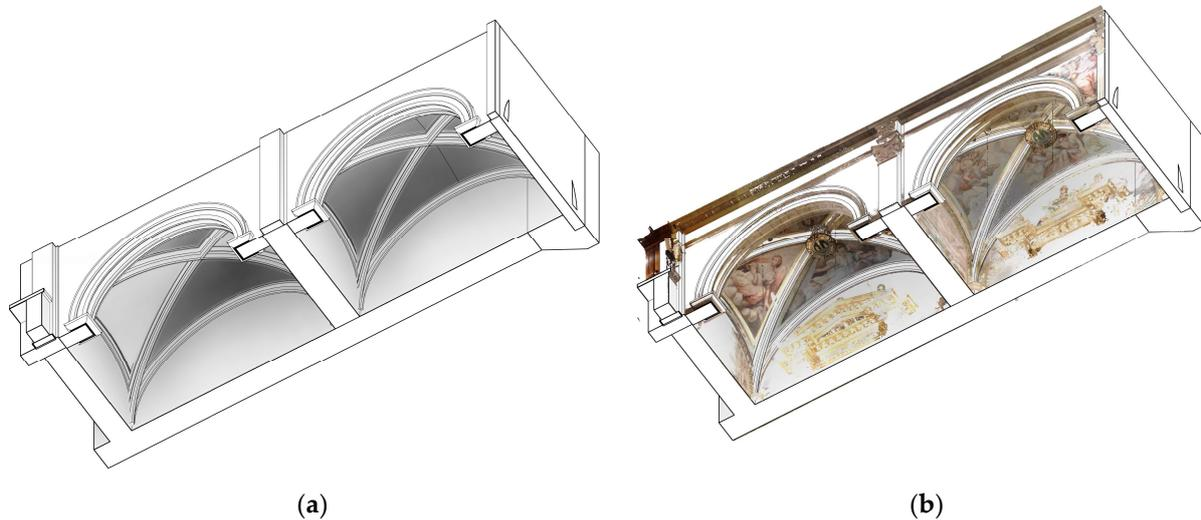
**Figure 5.** (a) Bottom view of the modelling of the vaults using the mass tool; (b) bottom view of the modelling of the vaults using the mass tool with the point cloud overlay. Source: own elaboration (2024).
