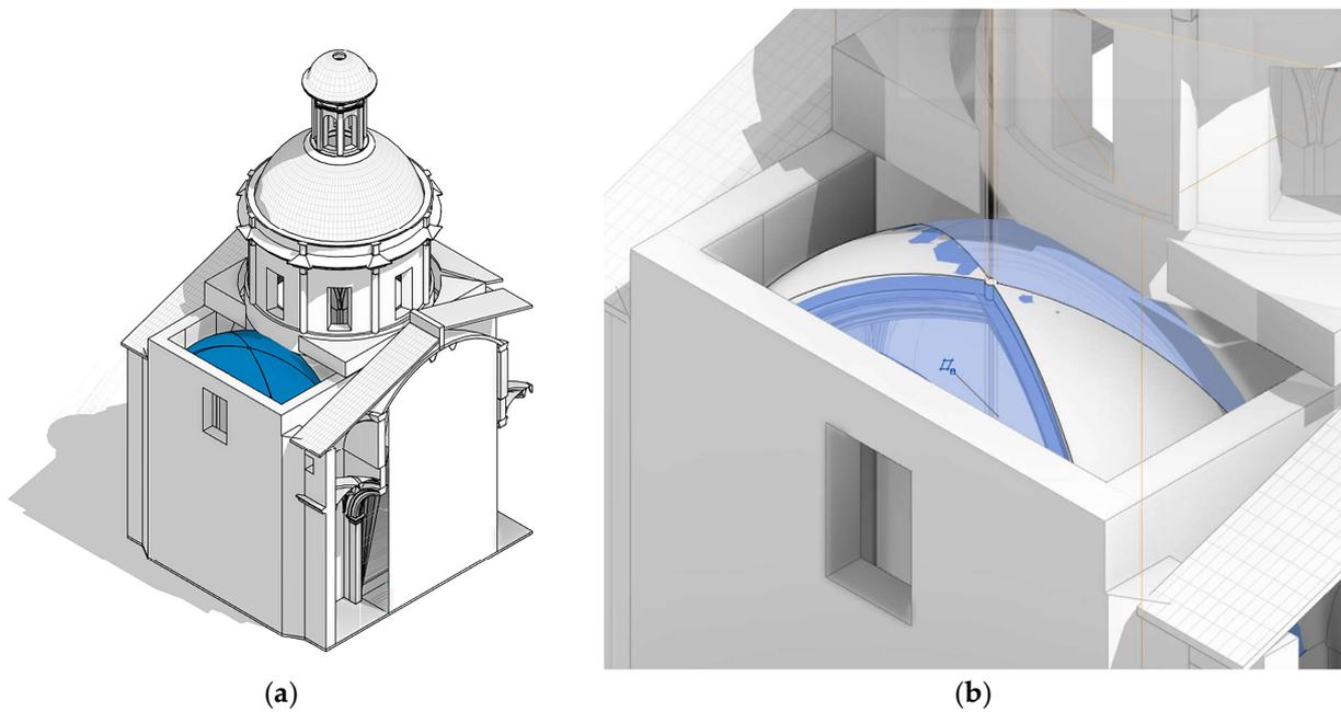
**Figure 11.** In blue: modelling of the plementeries separately and within a group (a); detail of the modelling of the plementeries facing each other and the small circumference made at the junction of the plementeries (b). Source: own elaboration (2024).
