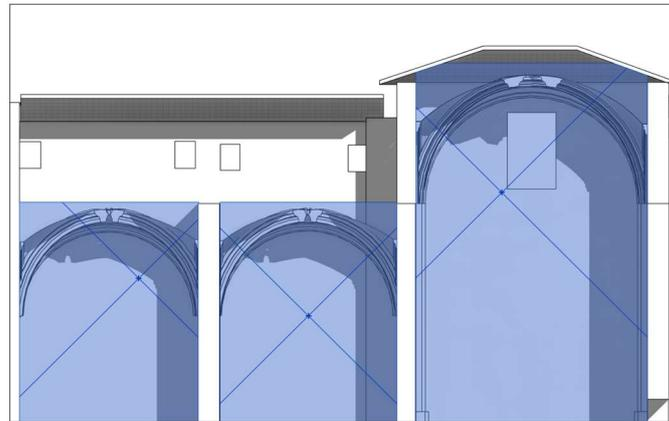
**Figure 7.** Visualisation of the vaults using the 2D section in Revit 2024, demonstrating that the height of the spaces is not constrained by the mass surfaces generated. Source: own elaboration (2024).
