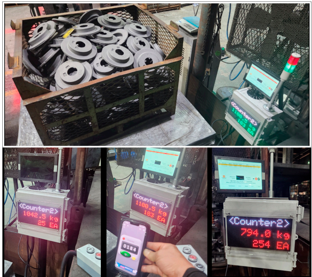
Figure 10. Images of the test result showing the product counting accuracy.
