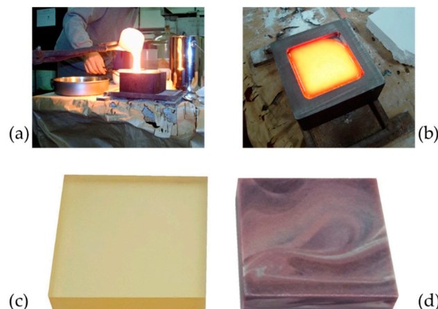
Figure 1. Casting of the parent glass (a,b); specimen before (c) and after (d) crystallization treatment.
