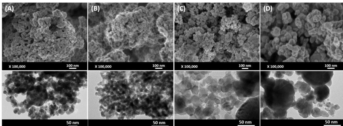
**Figure 3.** SEM (top) and TEM (down) images of the as-detonated (A)  $CeO_2$ , (B)  $HfO_2$ , (C)  $Nb_2O_5$ , and (D)  $In_2O_3$  oxide ceramics, respectively.
