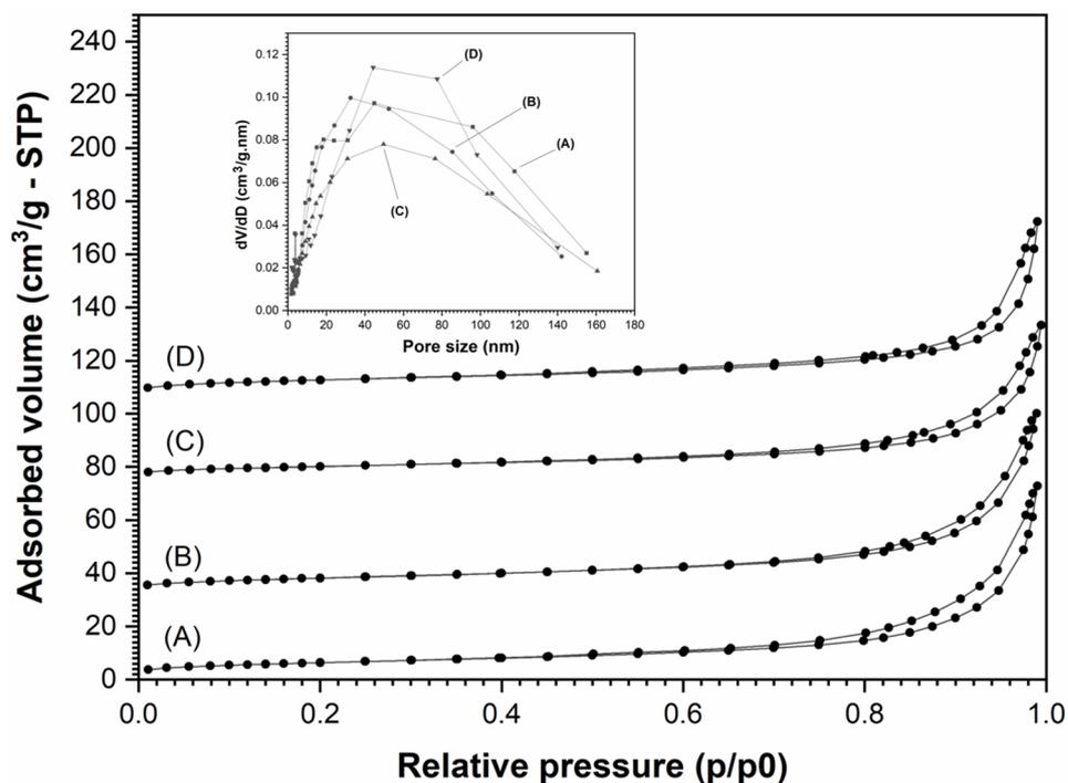
**Figure 4.** Nitrogen isotherms of the as-detonated ceramics: (A) CeO<sub>2</sub>, (B) HfO<sub>2</sub>, (C) Nb<sub>2</sub>O<sub>5</sub> and (D) In<sub>2</sub>O<sub>3</sub> materials, respectively. In the insert, the corresponding particle size distributions.
