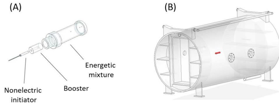
**Figure 1.** The energetic train (A) and the detonation chamber (B) used for the synthesis of oxide ceramics. The red cylinder in the detonation chamber represents the energetic train.
