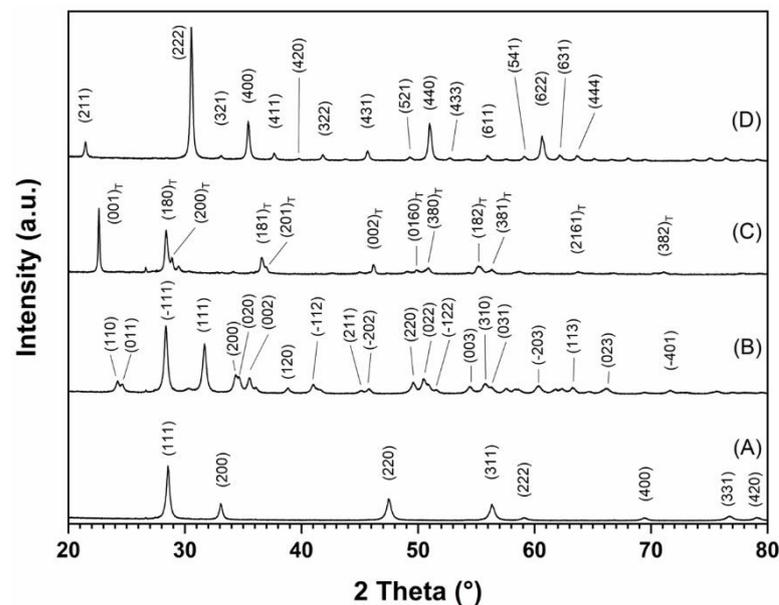
**Figure 2.** XRD patterns of the as-detonated oxide ceramics: (A)  $\text{CeO}_2$  (JCPDS card No. 01-081-0792), (B)  $\text{HfO}_2$  (JCPDS card No. 00-034-0104), (C)  $\text{Nb}_2\text{O}_5$  (JCPDS cards No. 00-30-0873), and (D)  $\text{In}_2\text{O}_3$  (JCPDS card No. 00-006-0416), respectively.
