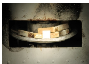
Figure 3. The sample of the material II after exposure to concentrated solar radiation.
