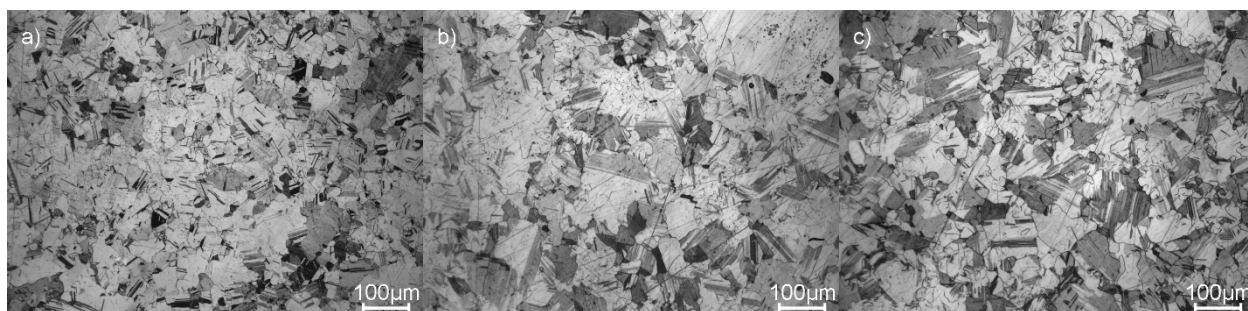
Figure S1. Images of the polished and etched surfaces of the original ZnSe samples from different manufacturers: the polycrystalline ZnSe manufactured by INOPTICS, Nizhny Novgorod, Russia (a); the polycrystalline ZnSe manufactured by PromLab LLC, Nizhny Novgorod, Russia (b); the polycrystalline ZnSe manufactured by II-VI Incorporated, Saxonburg, USA (c).
