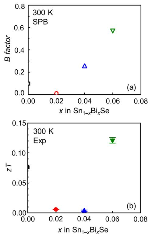
**Figure 4.** (a) Calculated  $B$ -factor varying with  $x$  in  $\text{Sn}_{1-x}\text{Bi}_x\text{Se}$  ( $x = 0.00, 0.02, 0.04, \text{ and } 0.06$ ) at 300 K, (b) experimental  $zT$  varying with  $x$  in  $\text{Sn}_{1-x}\text{Bi}_x\text{Se}$  ( $x = 0.00, 0.02, 0.04, \text{ and } 0.06$ ) at 300 K [18].
