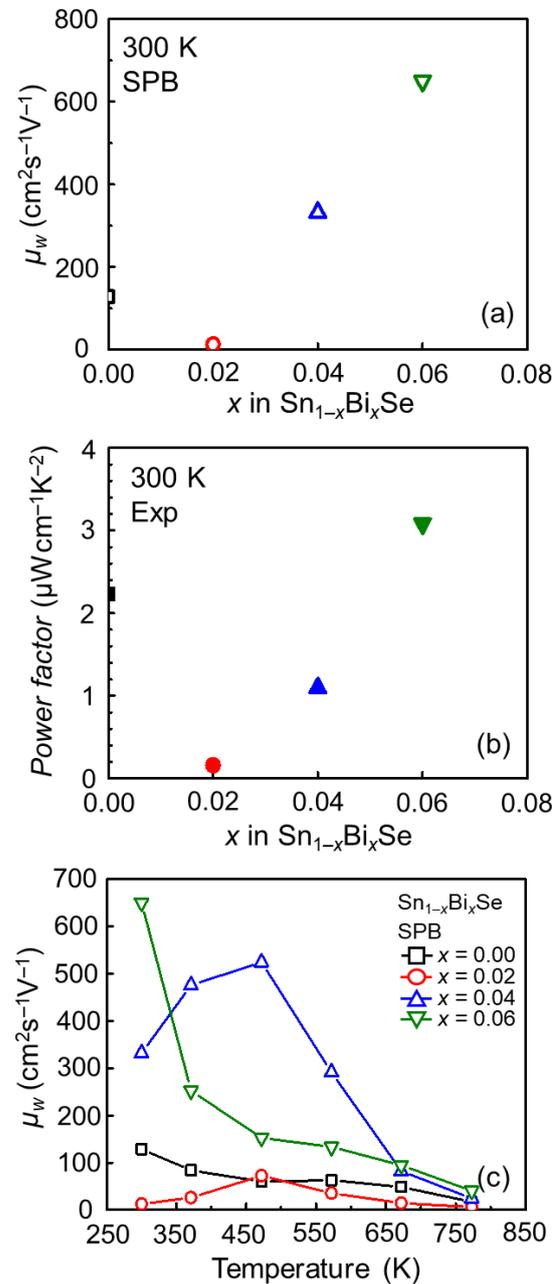
**Figure 3.** (a) Calculated weighted mobility ( $\mu_W$ ) varying with  $x$  in  $\text{Sn}_{1-x}\text{Bi}_x\text{Se}$  ( $x = 0.00, 0.02, 0.04$ , and  $0.06$ ) at 300 K, (b) experimental power factor varying with  $x$  in  $\text{Sn}_{1-x}\text{Bi}_x\text{Se}$  ( $x = 0.00, 0.02, 0.04$ , and  $0.06$ ) at 300 K [18], and (c) calculated  $\mu_W$  for  $\text{Sn}_{1-x}\text{Bi}_x\text{Se}$  ( $x = 0.00, 0.02, 0.04$ , and  $0.06$ ) varying with temperature (300–773 K).
