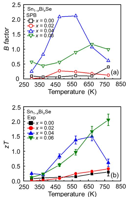
**Figure 5.** (a) Calculated temperature-dependent  $B$ -factor varying with  $x$  in  $\text{Sn}_{1-x}\text{Bi}_x\text{Se}$  ( $x = 0.00, 0.02, 0.04,$  and  $0.06$ ), (b) experimental temperature-dependent  $zT$  varying with  $x$  in  $\text{Sn}_{1-x}\text{Bi}_x\text{Se}$  ( $x = 0.00, 0.02, 0.04,$  and  $0.06$ ) [18].
