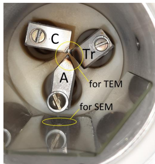
Figure 5. The appearance of the discharge assembly and the glass substrate after 7200 discharge pulses.
