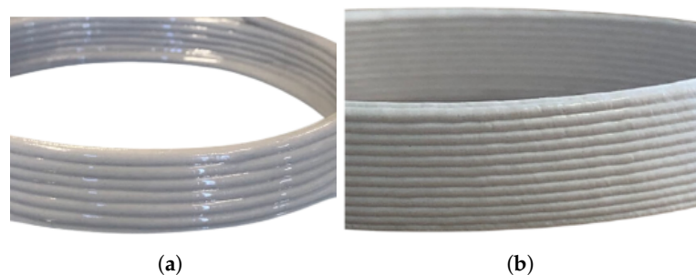
Figure 17. Printing of cylindrical geometry: (a) printing with a nozzle of 2 mm; (b) printing with a nozzle of 0.6 mm.
