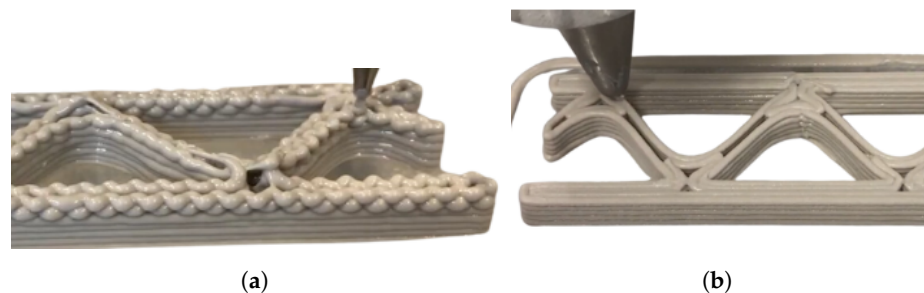
Figure 18. Complex shape printing: (a) wavy patterns; (b) conforming part.
