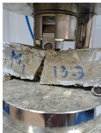
Figure 7. Flexural strength test.
