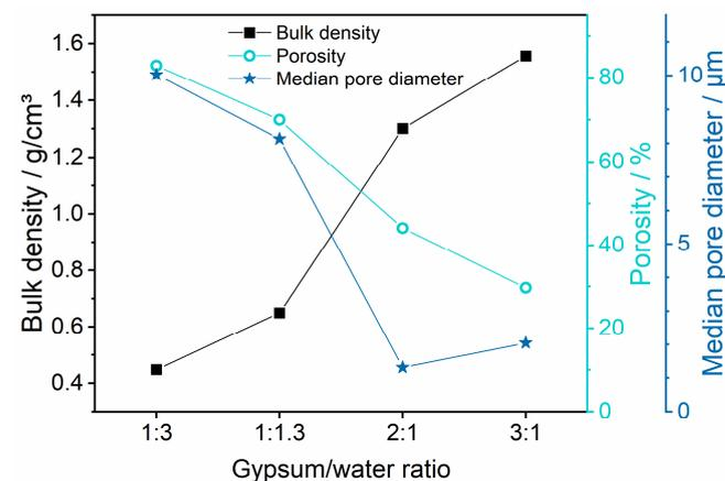
**Figure 1.** Bulk density, porosity, and median pore opening diameter of plaster mould materials prepared from varying gypsum/water ratios, determined via mercury intrusion porosimetry.
