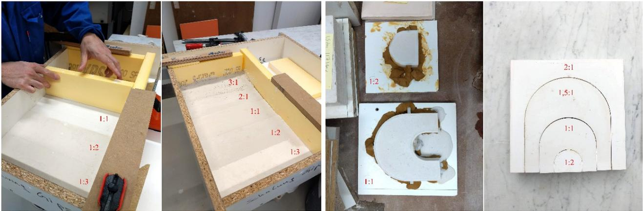
**Figure 10.** Production process for the two gradient plaster moulds. **Left:** Linear gradient mould produced by subsequent casting of parts with various densities in one master mould. **Right:** Radial gradient mould produced by combining four individual parts with different densities.
