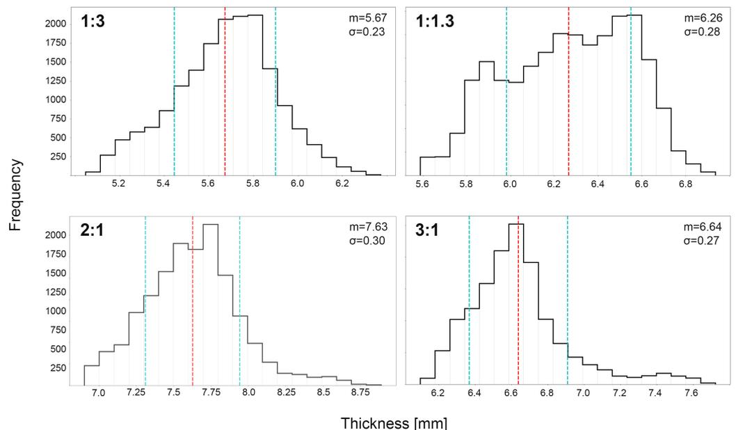
**Figure 7.** Thickness values distribution in mm of the 4 fired clay samples ( $75 \times 75$  mm<sup>2</sup>) extracted from 3D point cloud data. The mean thickness values (red) of the samples range between a minimum of 5.67 mm in mould 1:3 and a maximum of 7.63 mm in mould 2:1. Standard deviation values (blue) quantify the variability in thickness distribution across the samples' surface in a range between  $\pm 0.30$  mm in mould 2:1 and  $\pm 0.23$  in mould 1:3.
