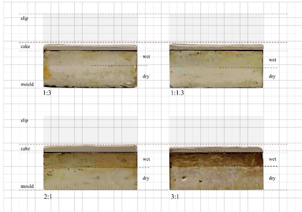
**Figure 6.** The four plaster moulds with various densities with their corresponding clay cakes in wet green state. The depth of the water absorption of the moulds is indicated with a dashed line and is divided into wet and dry. The slip level during casting is highlighted with grey colour. Casting duration 60 min. Square grid represents 1 cm.
