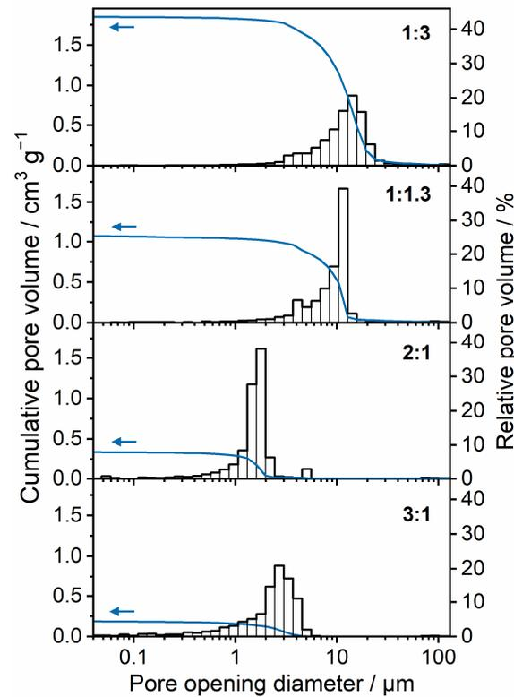
**Figure 2.** Pore opening diameter distribution of plaster mould materials prepared from varying gypsum/water ratios, determined via mercury intrusion porosimetry.
