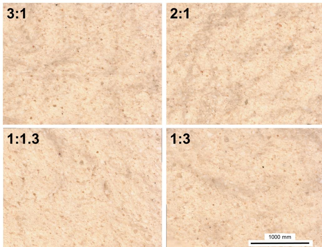
**Figure 4.** Light optical micrographs of fracture surfaces of fired clay samples cast in plaster mould materials prepared from varying gypsum/water ratios.
