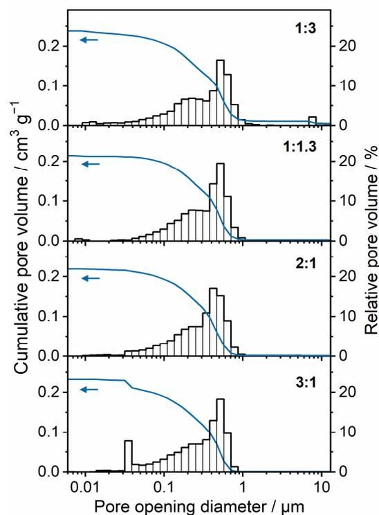
**Figure 3.** Pore opening diameter distribution of fired clay samples cast in plaster mould materials prepared from varying gypsum/water ratios, determined via mercury intrusion porosimetry.
