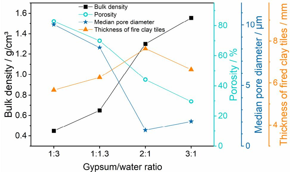
**Figure 8.** Bulk density, porosity, and median pore opening diameter of gypsum mould materials prepared from varying gypsum/water ratios, determined via mercury intrusion porosimetry, as well as the average thickness values of the respective clay casts after firing.
