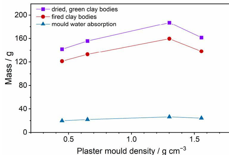
**Figure 5.** Correlation between plaster mould densities and cast/mould masses. Mass data of the four plaster clay casts of different G:W ratios (1:3, 1:1.3, 2:1, 3:1), in both dried green (purple line) and fired state (red line), as well as water absorption (blue line) of the four plaster moulds after the slip casting. Casting duration 60 min, casting area  $120 \times 120 \text{ mm}^2$ .
