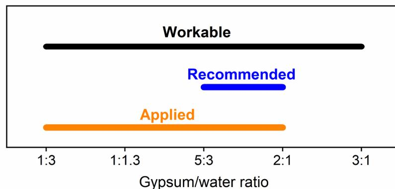
**Figure 9.** Ranges of gypsum/water ratios considered for plaster mould production. In black, the maximum workable range (higher or lower ratios resulting in excessively thick or thin plaster mixes). In blue, the recommended optimal range, as specified by the gypsum producer. In orange, the applied range ultimately utilised for the production of the thickness gradient (1:3 for the thinnest cake, 2:1 for the thickest).
