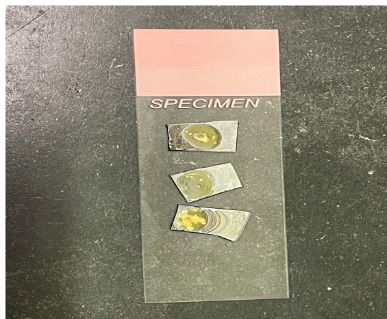
Figure 2. Deposits of polymerized sodium styrene sulfonate on silicon wafers.
