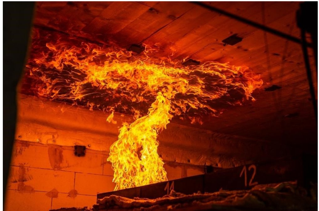
Figure 3. Flames from burner impacting ceiling in Experiment 3.
