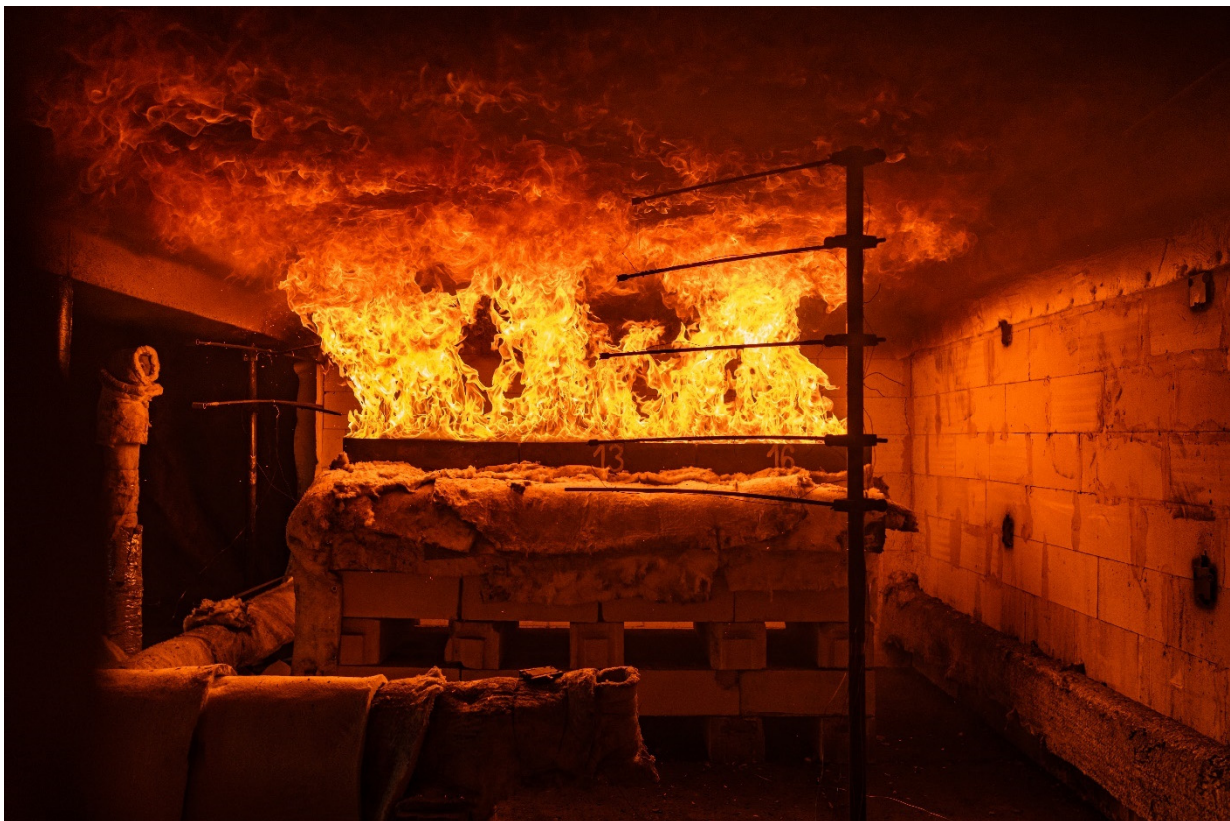
Figure 18. Flaming of the CLT ceiling in Experiment 3 during the 1250-kW steady phase.
