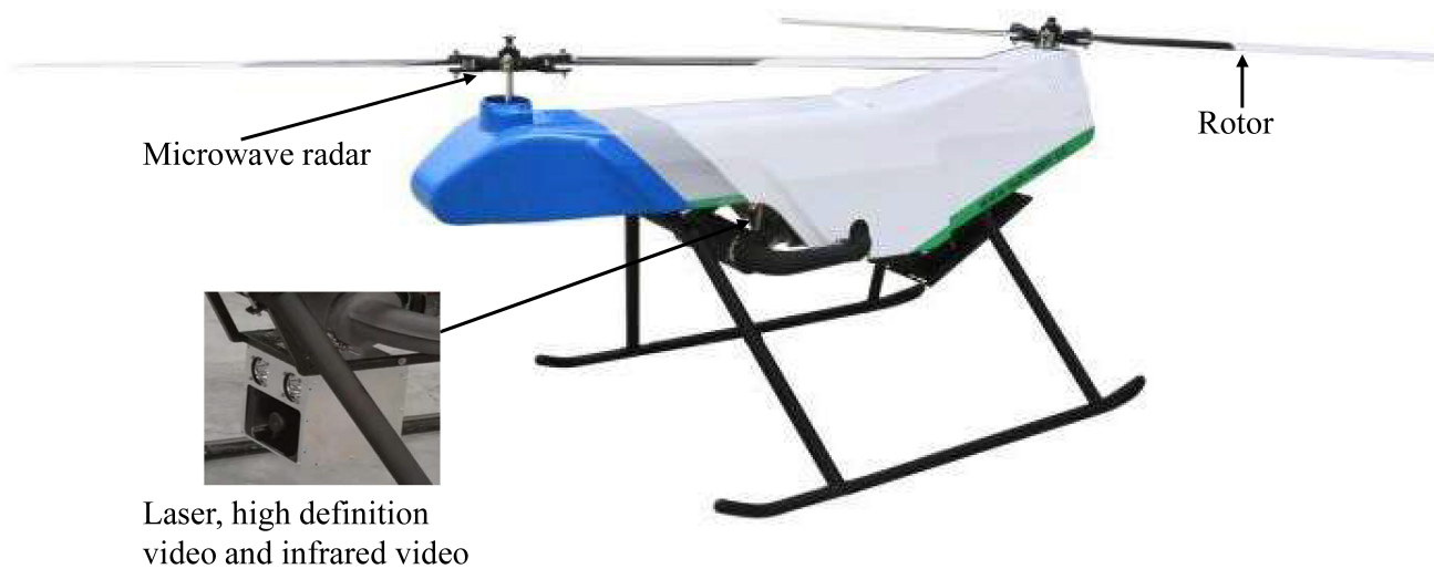
Figure 1. The drone used in LY100 fire extinguishing system.
