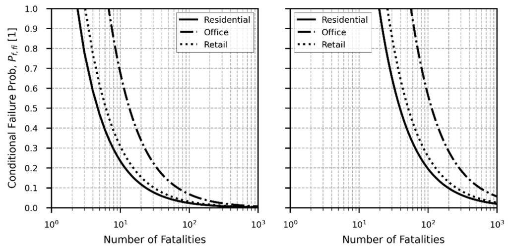
**Figure 6.** Conditional acceptable failure probability in the event of a structurally significant fire in function of the number of fatalities based on the principle of relative (marginal) lifesaving costs (**left**) without sprinklers, (**right**) with sprinklers.
