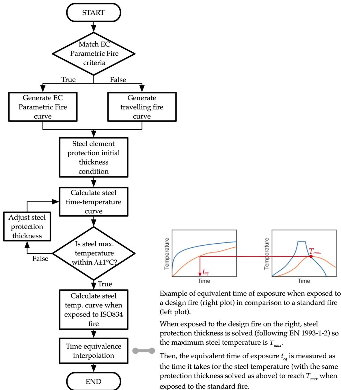
Figure 1. Simplified SFEPRAPY workflow for a single Monte Carlo simulation iteration.
