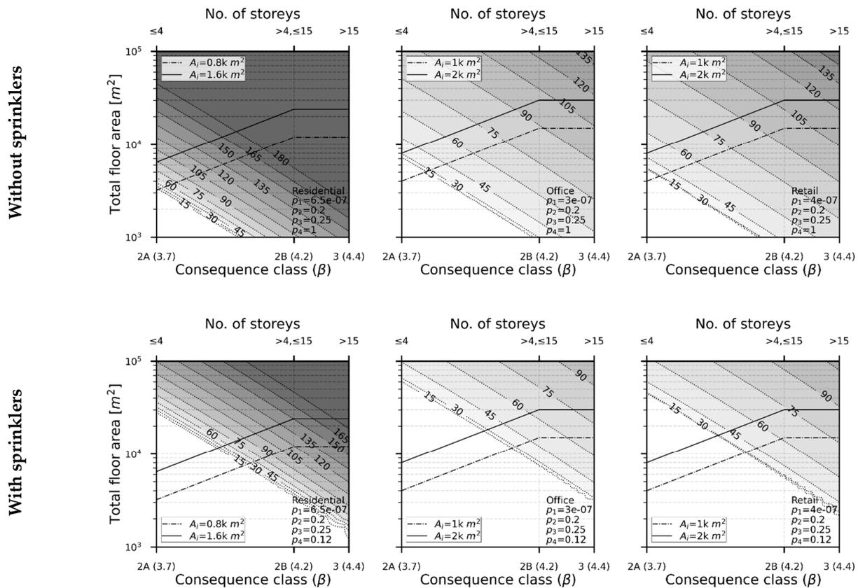
**Figure 3.** Contour plots of the solved structural fire-resistance rating at various building heights and total floor area (without and with sprinklers);  $A_i$  denotes floor area per storey.
