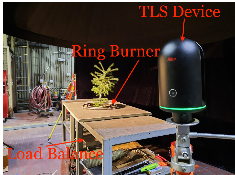
Figure 2. A labeled photograph of the experimental setup at the Missoula Fire Sciences Laboratory, illustrating the key components and their arrangement. The Terrestrial LIDAR Scanner is positioned to capture high-resolution point cloud data of the sapling, while the load balance measures the sapling's weight during the burning process. The ring burners provide controlled heat treatment, and an example sapling is shown in the testing area.
