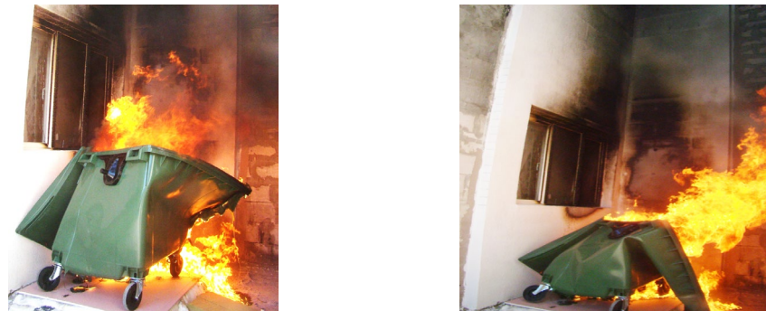
Figure 6. Containers start melting after 9:30 min.
