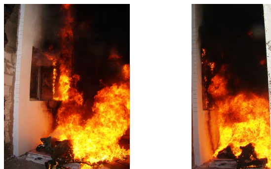
Figure 7. Fire penetration inside the room, after 14 min.
