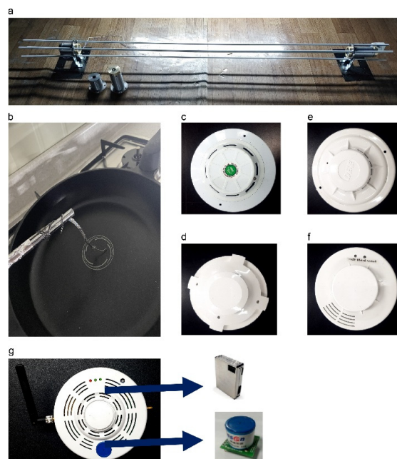
Figure 4. Measurement sensors: (a) optical density meter; (b) thermocouple; (c) manufacturer A (ASD); (d) manufacturer B (ASD); (e) manufacturer A (CSD) 15%; (f) manufacturer B (CSD) 15%; (g) indoor air quality sensor.
