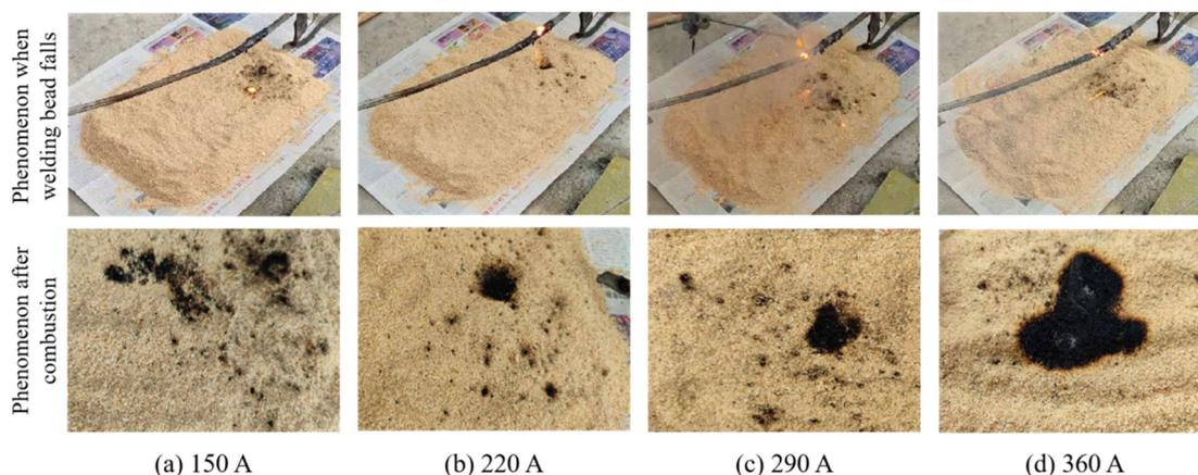
**Figure 12.** The ability of the welding spatters to ignite wood chips under different current intensities.
