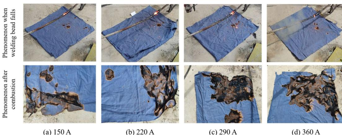
**Figure 11.** The ability of the welding spatters to ignite the cotton under different current intensities.
