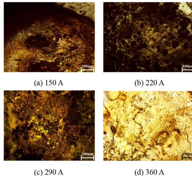
**Figure 13.** Microscopic image of the spatter magnified 50 times under different current intensities.
