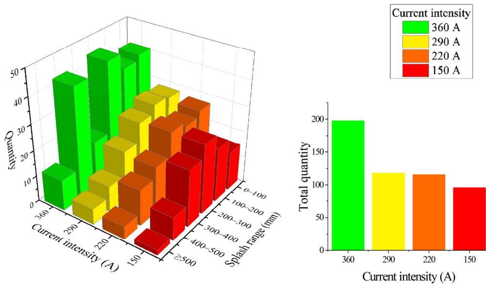
**Figure 3.** The quantity and the splash range of the spatters under different current intensities.
