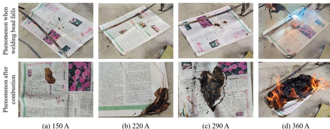
**Figure 10.** The ability of the welding spatters to ignite the newspaper under different current intensities.
