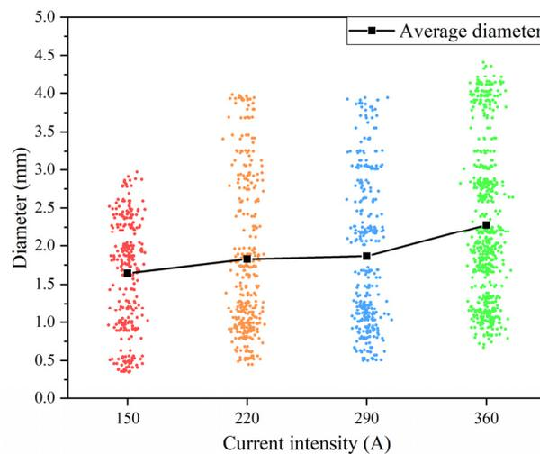
**Figure 4.** The distribution of the diameter of welding spatters.
