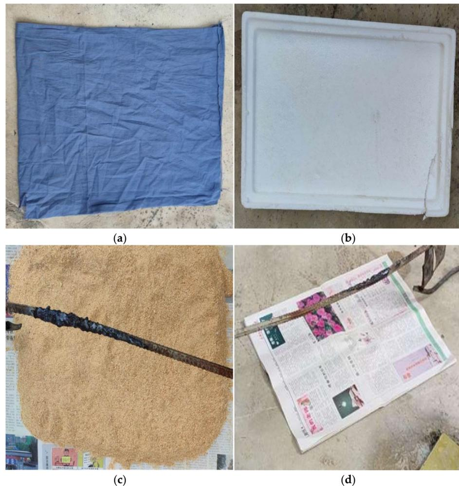
**Figure 1.** Ignition materials and their laying method. (a) Cotton. (b) Foam board. (c) Wood chip. (d) Newspaper.
