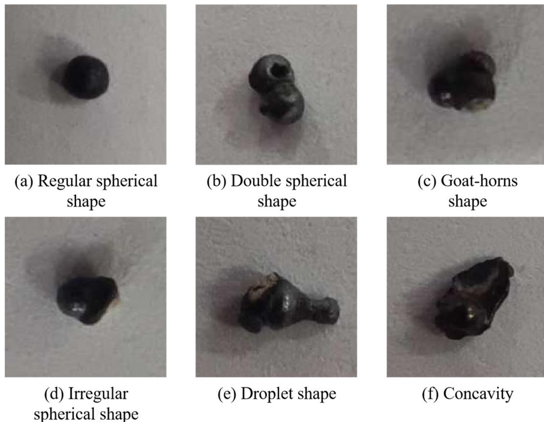
**Figure 5.** Shapes of welding spatters.
