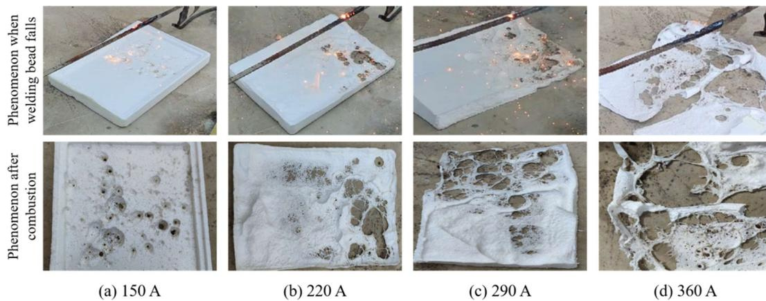
**Figure 9.** The ability of the welding spatters to ignite the foam board under different current intensities.
