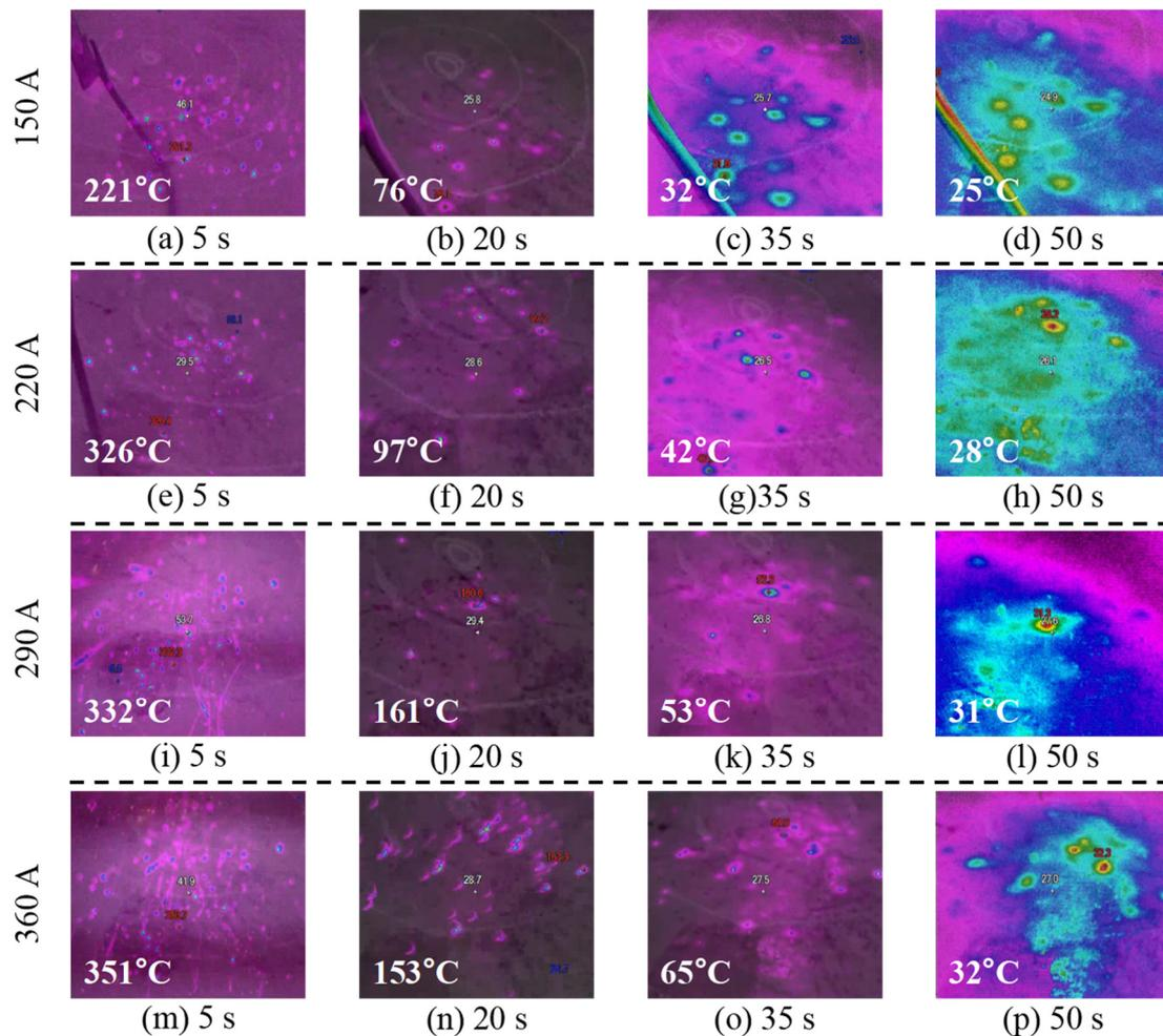
**Figure 7.** Infrared measurements of the temperature of the welding spatters under different current intensities.
