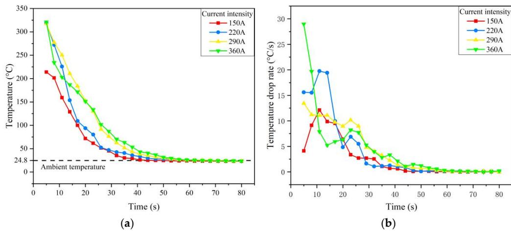
**Figure 8.** Temperature variation of the welding spatters with time at different current intensities. (a) Temperature curves under different current intensities. (b) Cooling rate curves under different current intensities.
