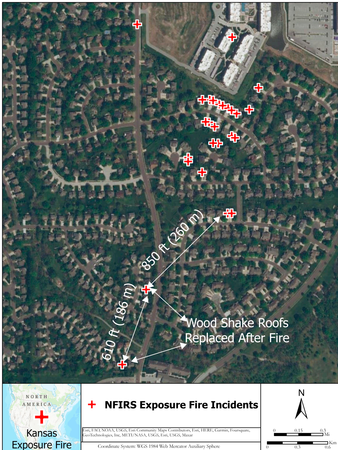
Figure 10. An NFIRS-documented exposure fire in Overland Park, Kansas on 20 March 2017. The exposure fire started in the apartment building at the north end of the map.
