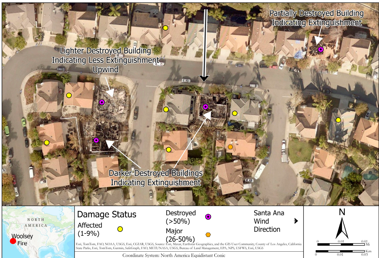
Figure 13. Indicators of defensive actions from Pictometry™ post-fire imagery [33] in a high-density area at the 2018 Woolsey Fire like homes with documented defensive actions in Figure 1. Partially burned buildings [35] with a darker appearance than their upwind [11] neighbors and damaged buildings, often adjacent to destroyed buildings [35], are established [15,16,26] indicators of defensive actions, further validated in this study.
