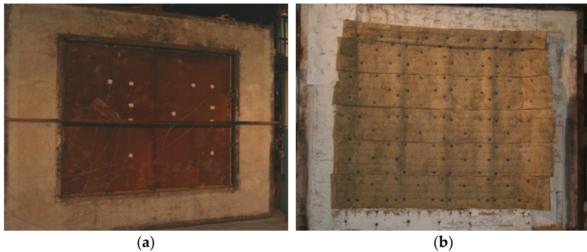
Figure 11. Bulkhead H-60 after testing on the heated (a) and unheated (b) side.
