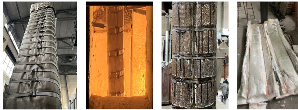
Figure 16. Non-combustible PROMIZOL-MIX PROPLATE system before, during, and after fire exposure (180 min) according to an S-curve fire.
