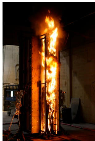
Figure 31. Cable tray fire. Refs. [181,182].
