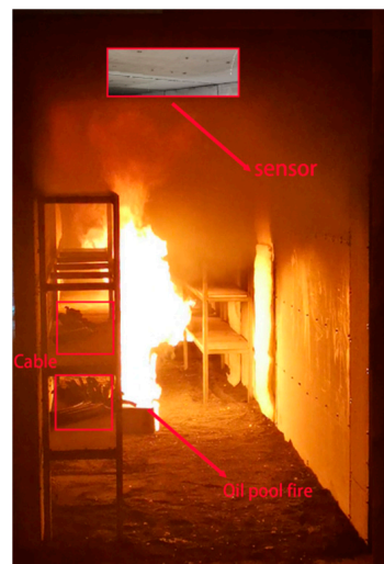
Figure 5. Square cable trench experimental platform.
