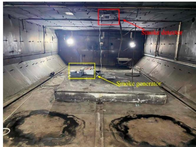
**Figure 13.** Layout of smoke detectors and experimental equipment in test cargo compartment.
