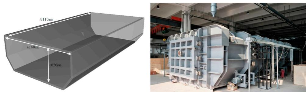
**Figure 12.** The aircraft cargo compartment ground simulation platform: the left image shows the dimensional diagram and the right image shows the actual photo.
