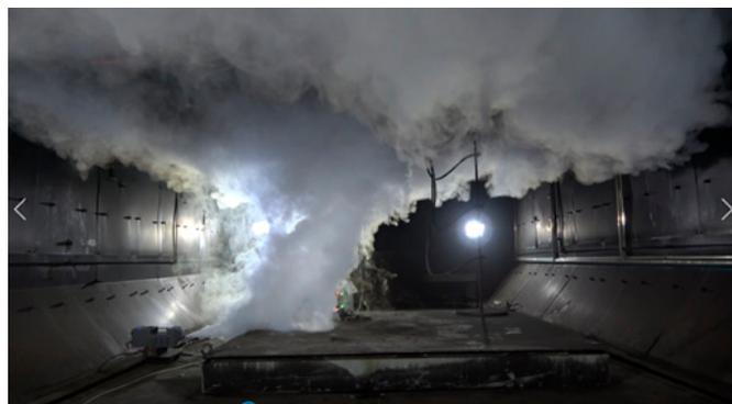
**Figure 14.** Smoke movement inside cargo compartment during experiment.
