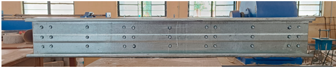
Figure 1. Beam sections connected using self-tapping screws [27].
