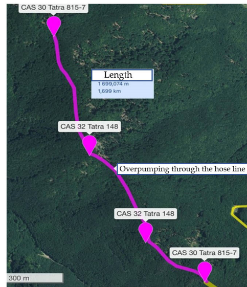
Figure 16. Water transport between 400 m distant sites up to the outlet hose [29].
