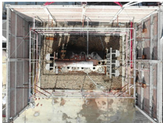
Figure 2. Fire model fact map of 220 kV oil-immersed transformer.
