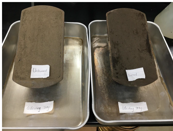
Figure 7. Original (unburned) and burned soil samples subjected to surface erosion. Note that the sample corresponding to a (room) temperature of 20 °C indicates the original unburned soil, the temperature of 400 °C indicates low-severity burn, 600 °C indicates moderate-severity burn and 800 °C and 1000 °C indicate high-severity burn.
