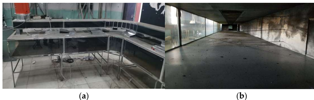
Figure 1. UTLT smoke control experimental platform. (a) Main structure of the platform; (b) internal structure of the platform.
