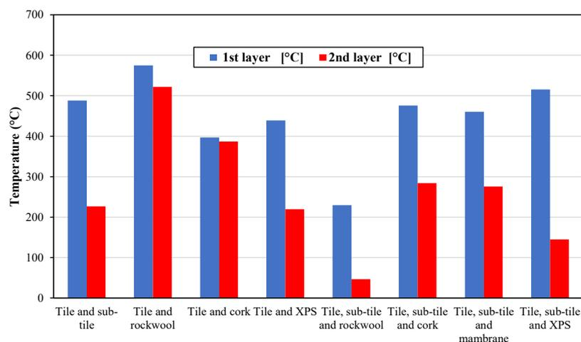
**Figure 6.** Maximum temperatures recorded in the 1st layer and 2nd layer for all roof specimens.
