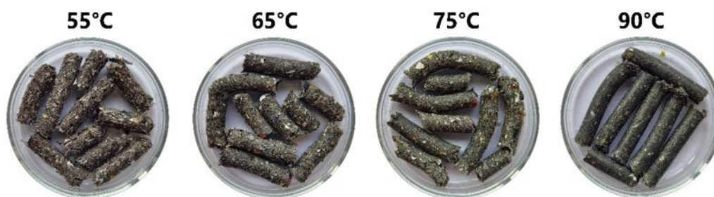
Figure 3. The produced SRF pellets for pelletising temperatures of 55 °C, 65 °C, 75 °C, and 90 °C.
